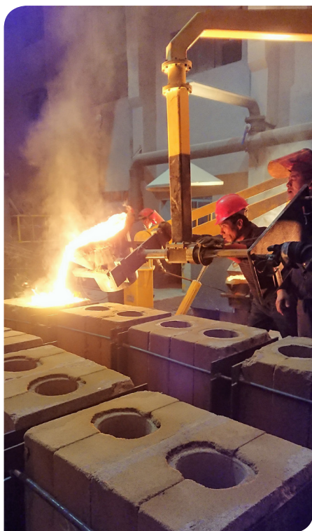
Above: Semi-automatic casting for bi-metal hammers.
